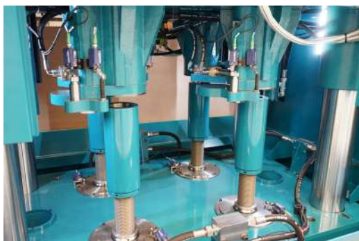
Clamping block system with multiple clamping points
