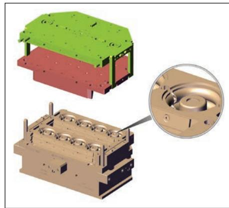
Fig. 3: Example of part (gas mask) with some undercuts and metallic inserts.
