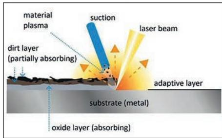
Fig. 5: Principle of the laser rotative head.
