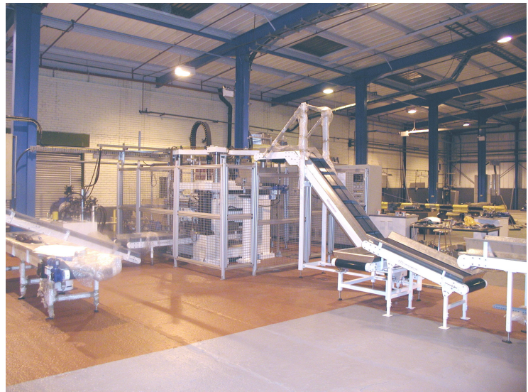
FIG. 6. – Typical 20 litre HSM production layout showing: (a) the HSM machine itself; (b) a typical factory setup with pre- and post-processing equipment
